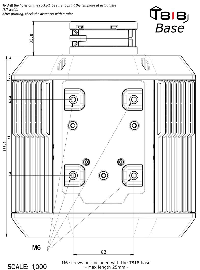
SCALE: 1,000 All dimensions are in millimeters
