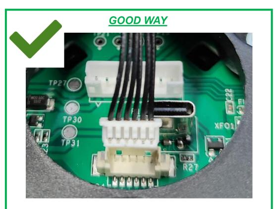
Take care to fully press-in the cable into connector.
