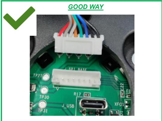
Take care to fully press-in the cable into connector.
