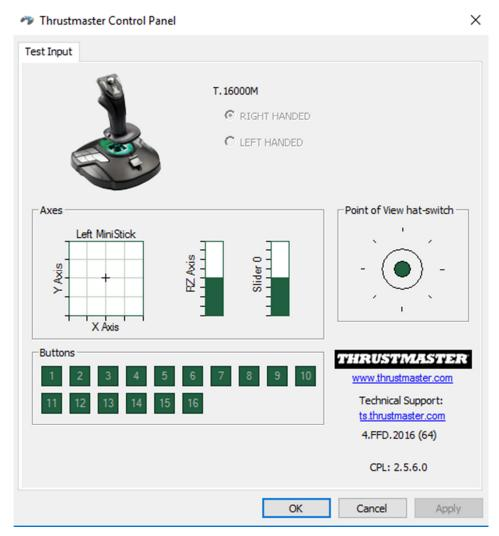
The bottom right corner of the Control Panel displays the information relative to your joystick and the drivers currently installed. Be sure to have this information at hand if you ever need to contact our technical support,
