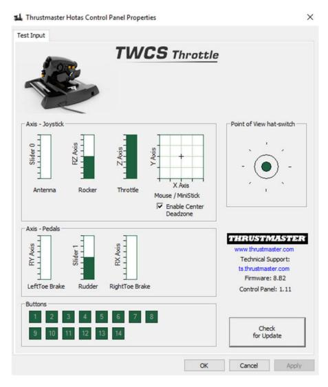
The bottom right corner of the Control Panel displays the information relative to your joystick and the drivers currently installed. Be sure to have this information at hand if you ever need to contact our technical support,
