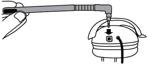
2. Make sure that the headset is properly connected to the Y Power Pack.
