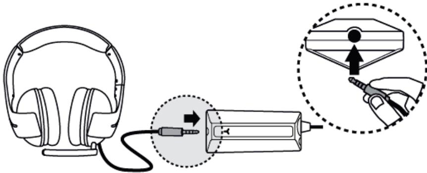
3. Make sure that the Y Sound Commander is properly connected to the Xbox One controller.
